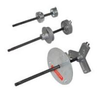
Make accurate, square cuts at floor level or in other blind locations. Easily present for depth of cut, they are installed in the pipe and make their cuts in seconds. Best used with individual PVC and ABS plastic pipe sizes ranging from 1 1/2" to 6" diameter.
