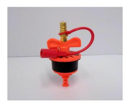
**The EXTRACTION-CAP** is a self-sealing vapor-sampling cap that takes the place of a standard monitoring well cap where vapor monitoring is required. It operates as a watertight locking expansion plug with the capability of having vapor or water extracted through the cap without removing the cap from the well. Quick connect attachment available.
